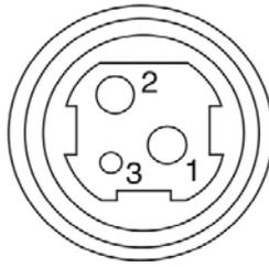
Figure 5-10 Power supply inlet
