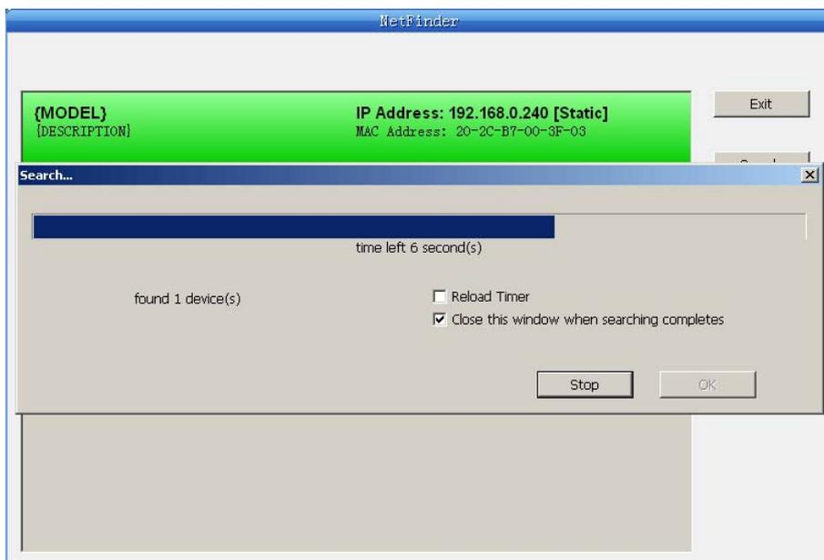
If the printer still can not be found out when the network connection is correct in the same network, Please check whether the network fire wall on the PC is open or not. If there is fire wall, please close it temporarily, open it again after finishing searching and setting a printer completely.
