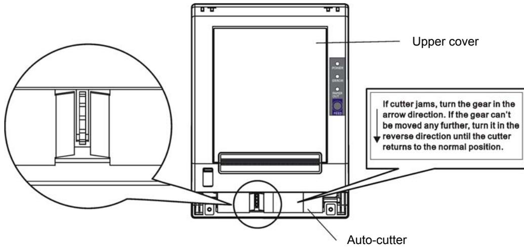
Figure 6-1 Adjust the auto-cutter by hand
