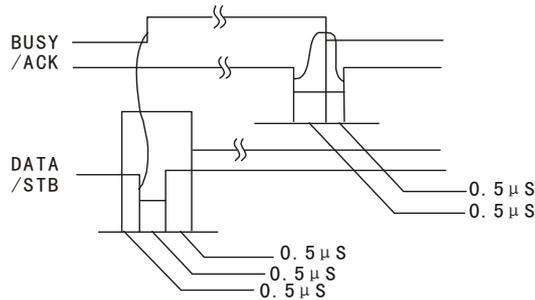
Figure 5-3 Timing signal of parallel interface
