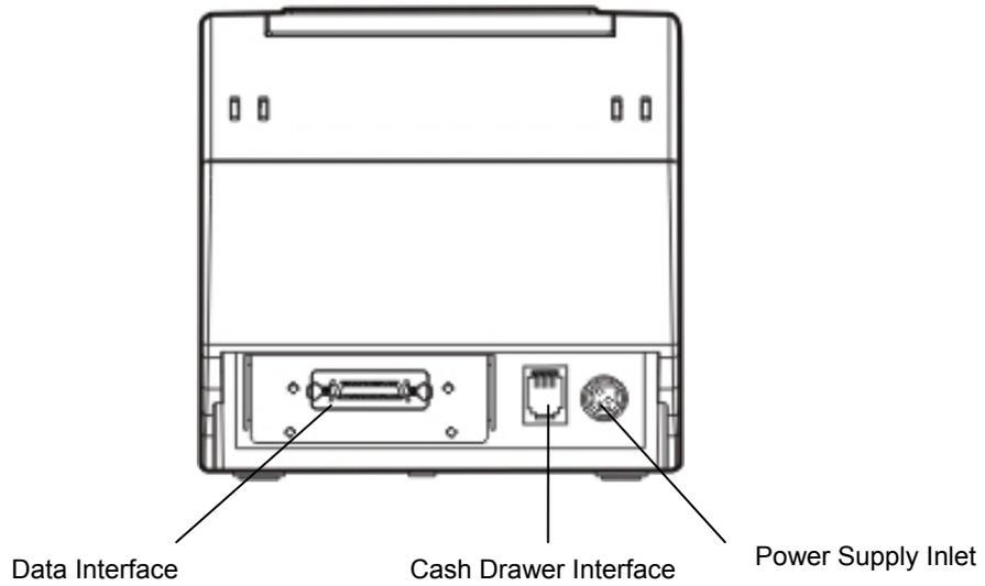
Figure 1-2 Interfaces on the back of the printer
