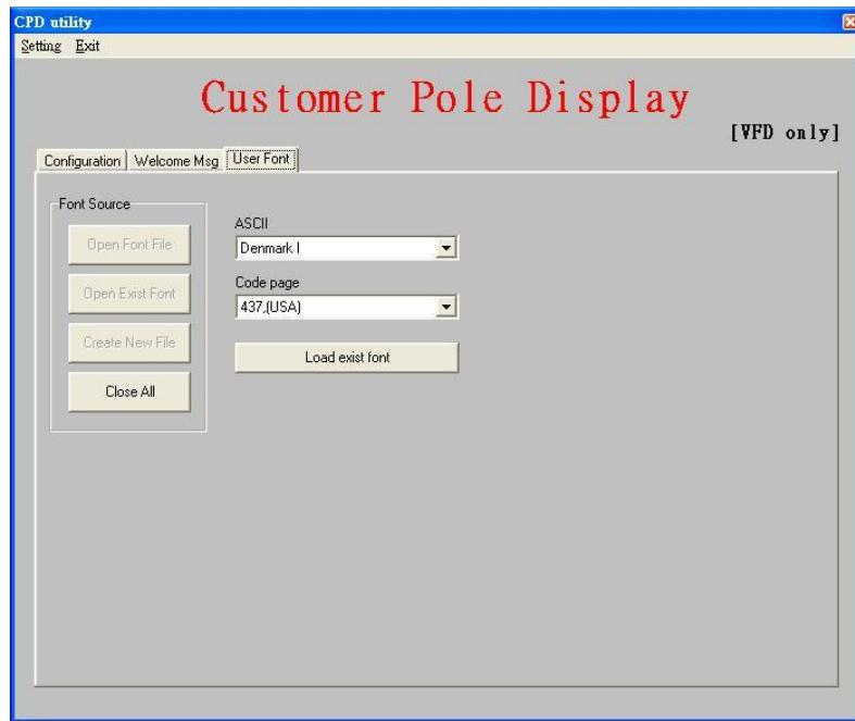
1, The first part is ASCII code which contains the characters coded as 0x20~0x7f. Within the ASCII, some of characters own different definition in different country. Please refer to the user's manual for the details of the code table.
