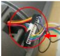
System connector supports PS/2 and RS-232 interface
