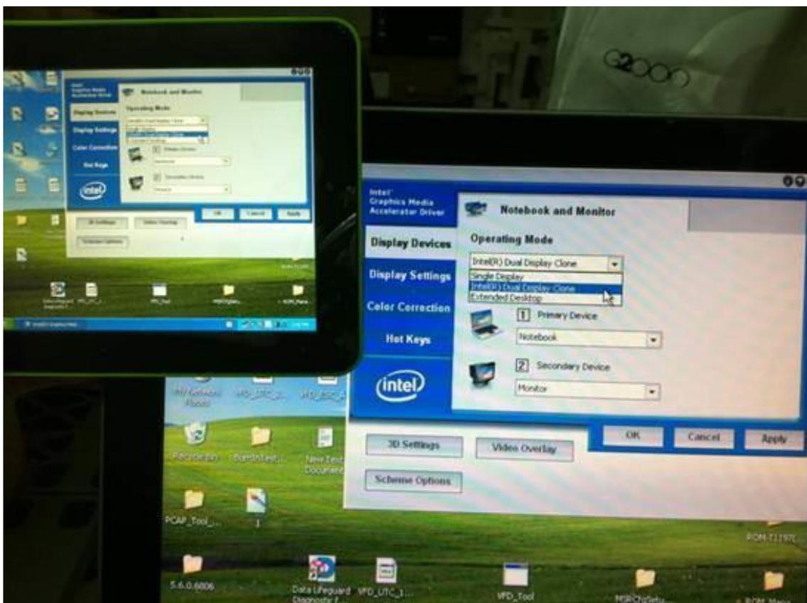
3. Extend mode, the resolution for main display is 1024\*768 and 2<sup>nd</sup> display is 800\*600.
