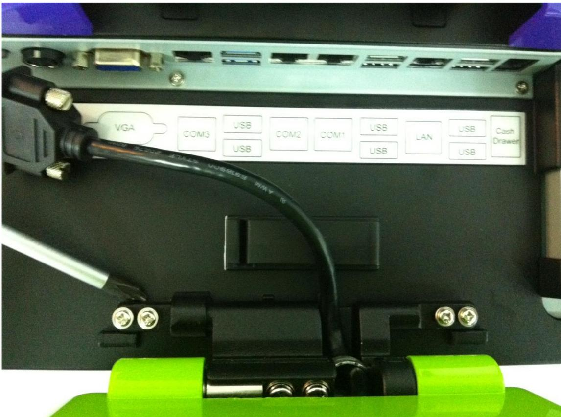
3. Plug the VGA cable to VGA port on the terminal.
